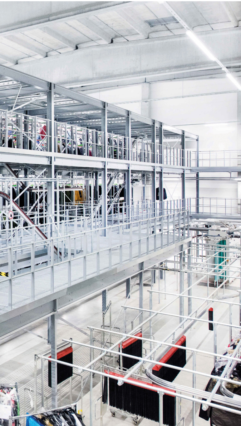
01 A hanging goods conveyor allows an automatic transport of garments between the levels of the hanging goods warehouse
