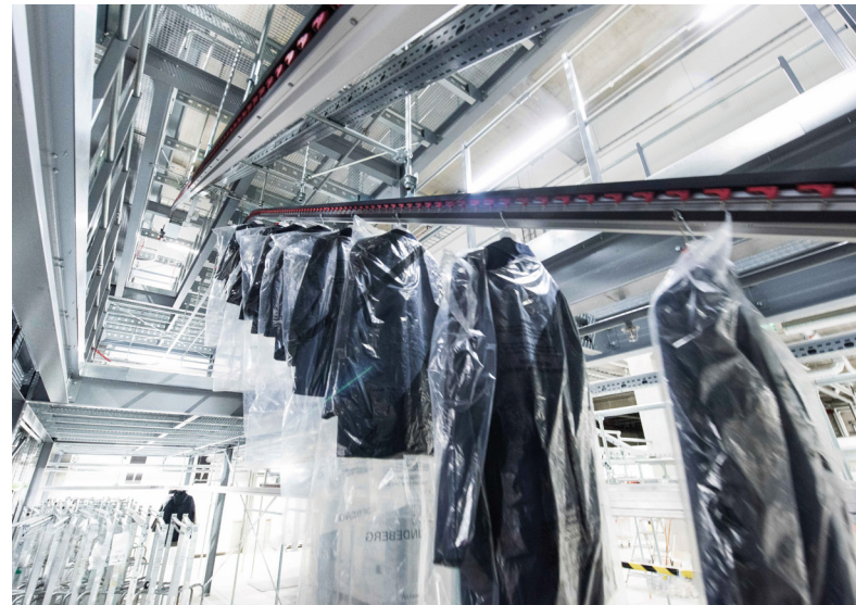
01 A hanging goods conveyor allows an automatic transport of garments between the levels of the hanging goods warehouse
