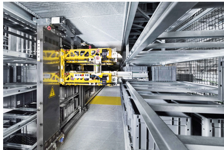
02 In the shuttle system, 72 multi-level shuttles, type Navette, store and retrieve up to four bins simultaneously
