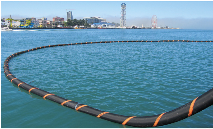
01 In the Batumi terminal in Georgia, highly resistant bunkering hoses from Continental transport fuel oil, carburetor fuels, and hot asphalt to and from the ships
