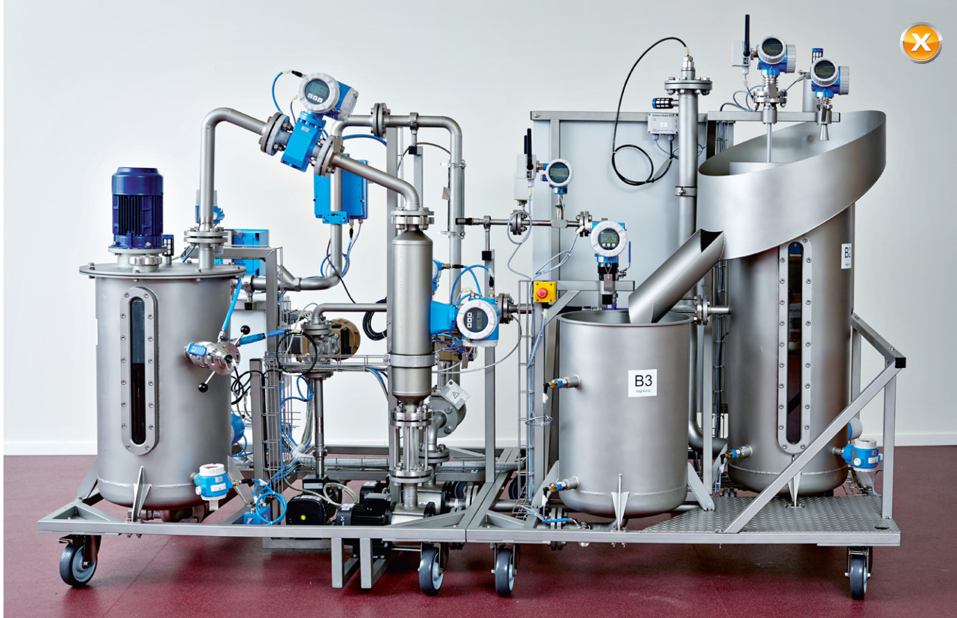
Endress+Hauser training rig provided to the Lao-German Technical School
