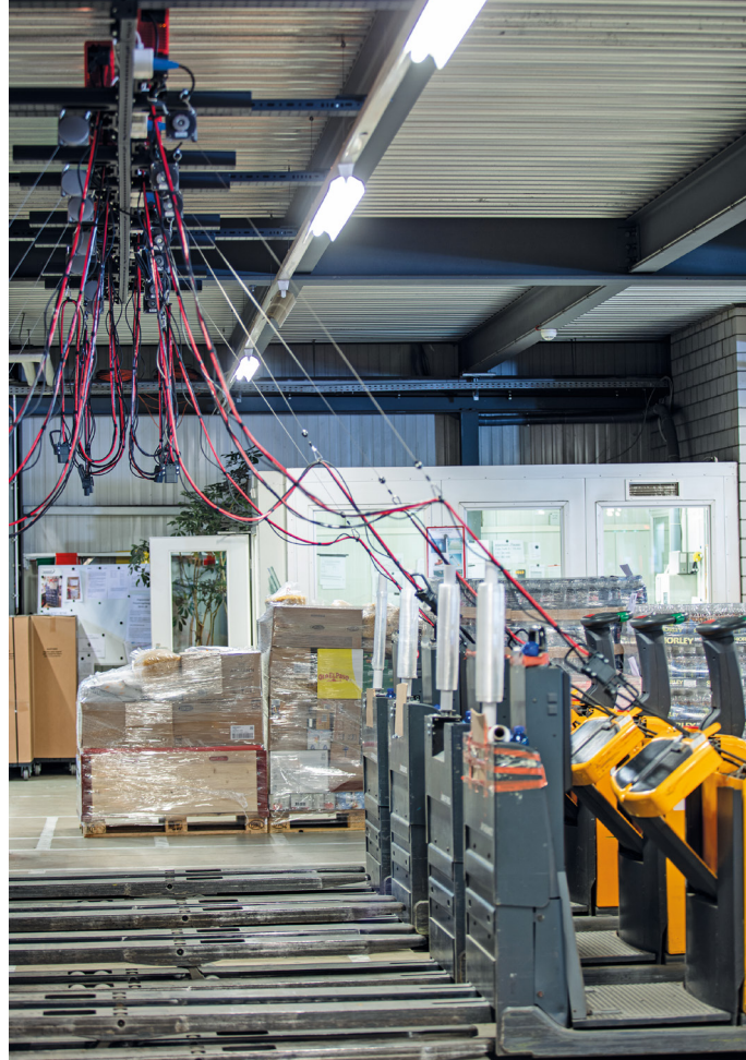
02 A spring balancer ensures that charging cables do not rest on the floor when not connected to a battery
