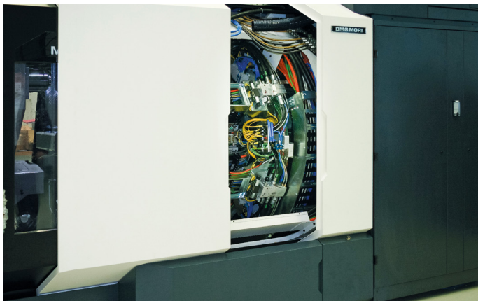
01 A look into the Multisprint shows the complex energy supply system from igus, completely mounted on the spindle drum of the machine
