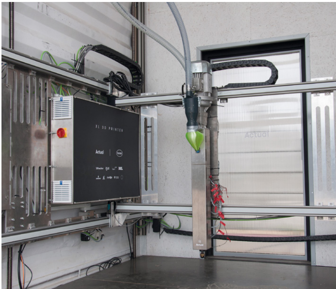
02 Insides of the mobile 3D printer; The print head moves on a drylin axis with toothed belt drive
