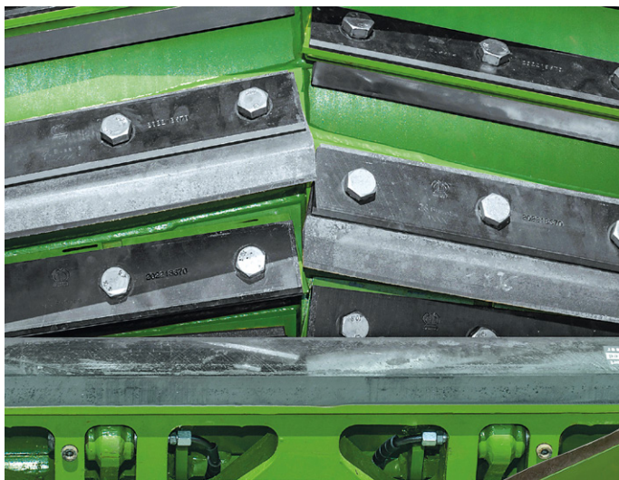
02 Chopping drum with shear blade
