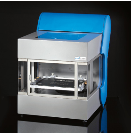
01 The EVOLizer prints based on the fused filament fabrication process (FFF). Thermoplastic fibres are melted and applied in layers
