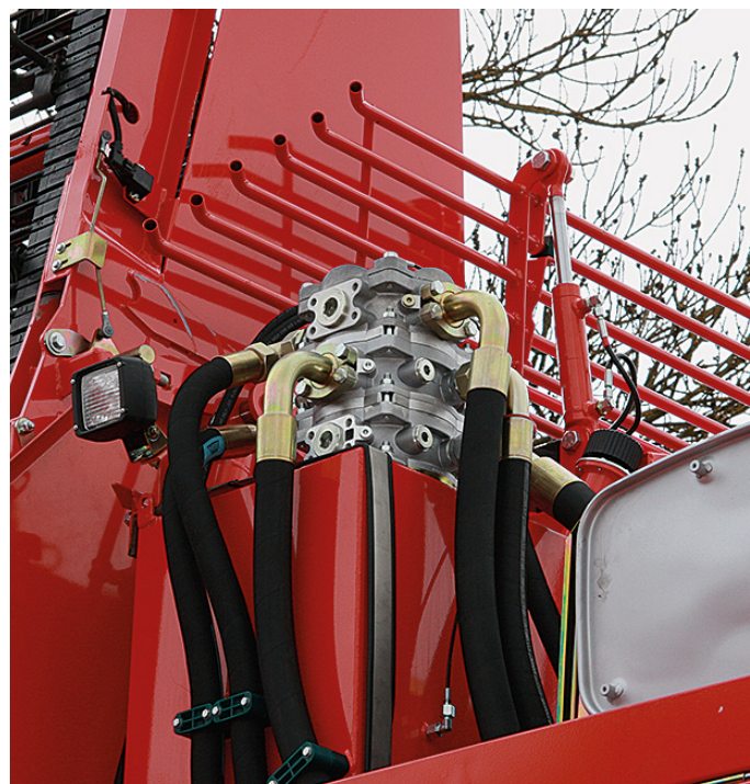
03 The above picture shows the return-suction filter with three connecting plates. All lines could be guided and directly connected to the filter. Just as uncomplicated, a housing ventilation was integrated in the filter cover
