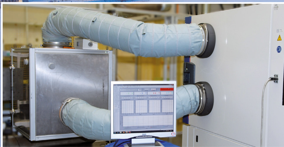
01 The EAS element clutch was successfully tested on an inertia dynamometer at low temperatures and harsh operating conditions
