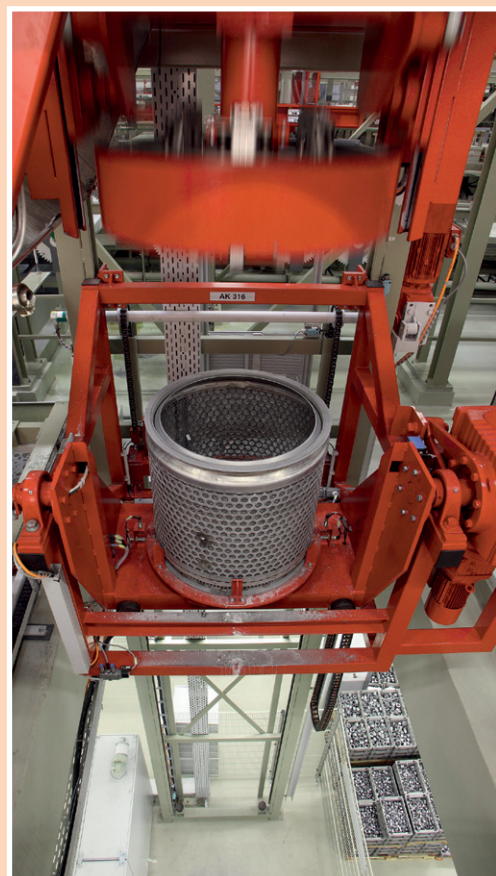
02 Smaller parts with internal threads are placed in drums for the coating process
