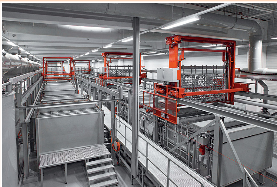
03 The inhouse electroplating plant is one of Europe's most modern plants and is specially designed for the various internal coating process stages – a degree of specialisation that would have been impossible with outsourcing
