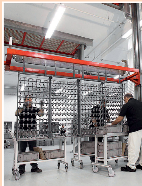
01 Larger coupling parts with weights of up to 2.5 kg and easily-damaged external threads are put on the racks manually in order to prevent potential damage during the coating process
