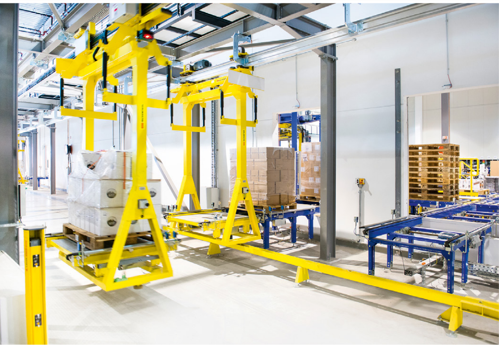
02 The monorail system circulates to all storage and picking areas
