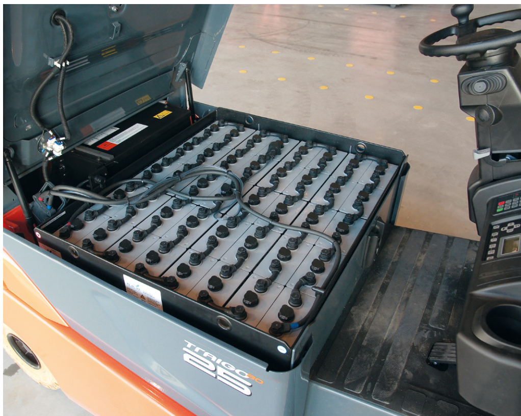
01 The forklift guarantees long operating periods with the 775 Ah/80 V battery on board
