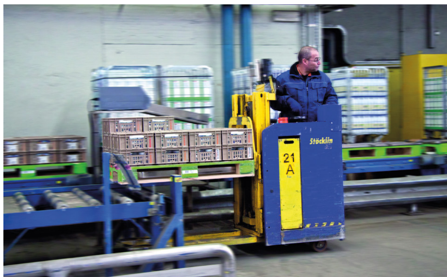
01 Type ESI 1600 electric platform stacker loading a pallet at the conveyor system
