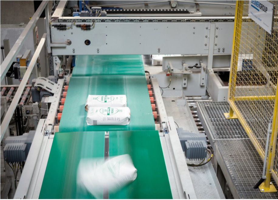
02 The twin-belt turning device: Two parallelly driven belt conveyors, which are driven with different speeds during the turning process, bring the bags gently into the required position
