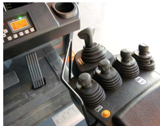
03 The mini levers can be used to intuitively and accurately initiate the mast functions
