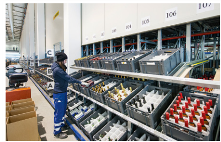
03 Picking of the fast-moving bottles with pick-by-voice
