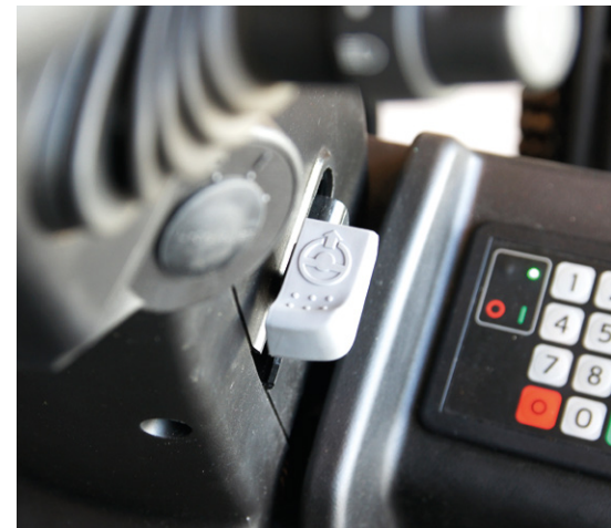
06 The memory function enables the steering column to return to the right position
