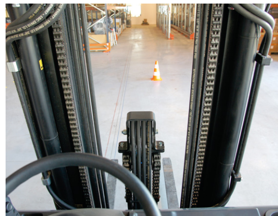
02 The wide design of the mast provides the driver with a good view of the load and fork
