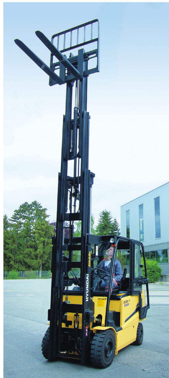
03 The counterbalanced forklifts are equipped with a complete driver's cab for outdoor use
