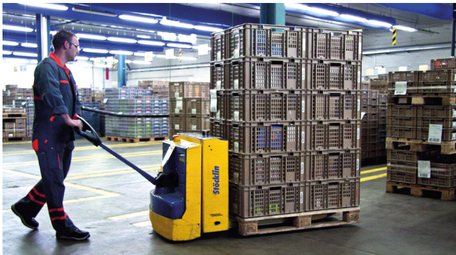
02 The ergonomically designed EDP 20 elevating transporters are used in the incoming goods department
