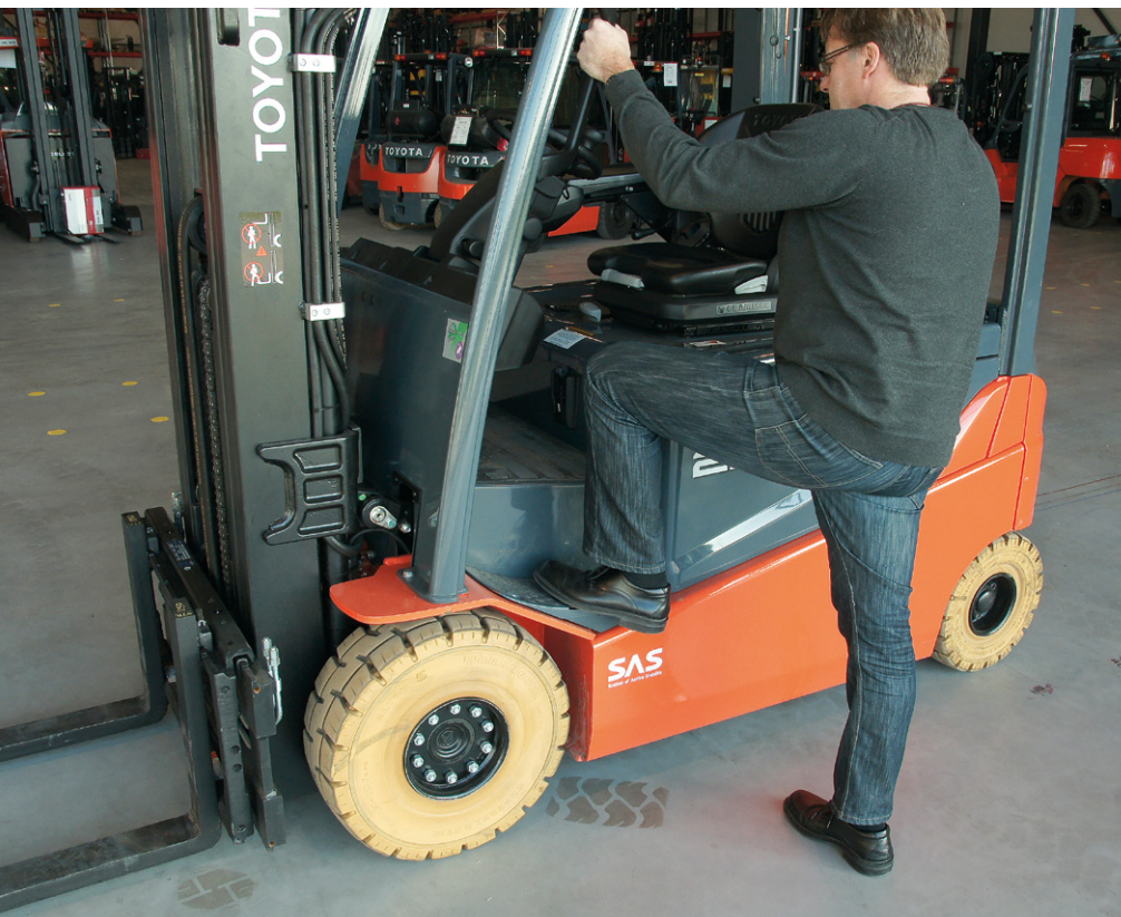
04 A smaller distance to the floor would certainly increase the comfort when getting on and off
