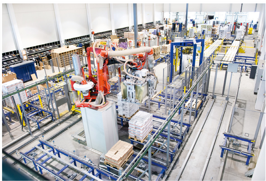
01 De-palletizing robots take off excessive heights and create new, storable pallets
